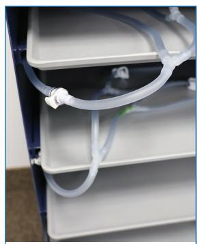
After sliding the endoscope tray into its tray slot, attach the tubing/adapter harness to the mainline quick connect fitting.
